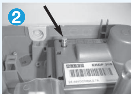
The pin descends into its housing
