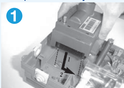
Fitting the motor
