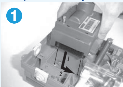
Fitting the motor
