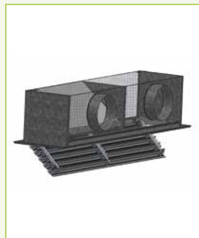
LINED Combined SO with plenum. Open position.
