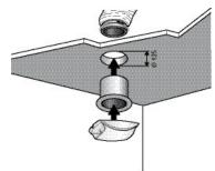
This grille is also very **easy to maintain**. Everything that gets dirty can be dismantled without removing the outlet: its **removable** front panel ease the access to the airflow regulator.
