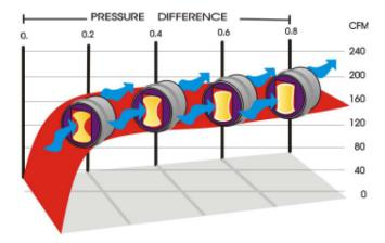
This curve illustrates the immediate action of a decreeing free area and increasing velocity resulting from increasing pressure to main constant airflow.
