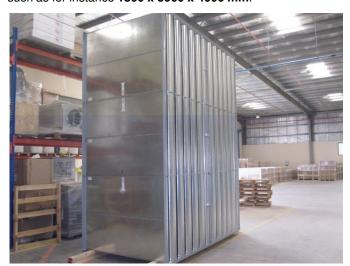
We had a requirement of approx. 16 nos. of sound attenuators with max. sizes of 900L x 4050W x 4050H for this project. The big challenge in the supply of these sound attenuators was to find a reliable supplier which could manage to manufacture as per these non-standard dimensions, in sections or in whole, without compromising on the quality of the silencers.
