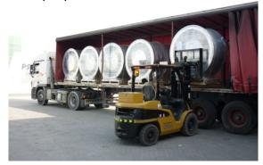
Circular sound attenuators can either be **passive** or **active**. In case of active sound attenuators, an electronics sensor is fixed on the outer casing that generates sound waves intended to cancel some of the noise generated by the fans in an HVAC system.
