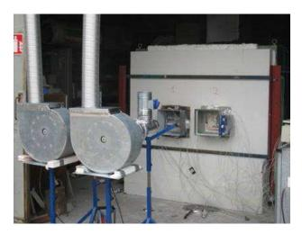
Damper 1 => UL 555 Classified damper (Model: FD 150CH – Aldes Middle East) Damper 2 => EN 1366-2 Certified damper (Model: ISONE - EM – Aldes France)
