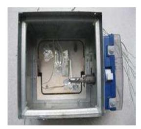
Thermocouples were installed on the blades as well as on the casing of each damper to measure temperature during the test.
