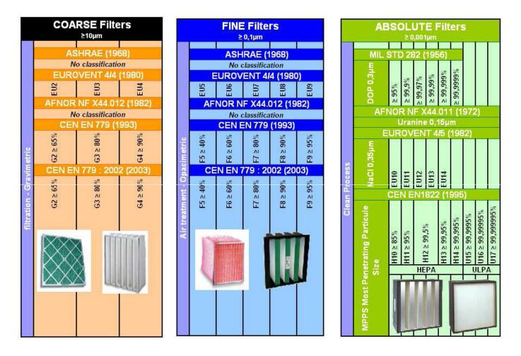
The filtration percentage indicated in this table corresponds with the percentage of particles (with the associated diameter) stopped by the filter. For example, a filter H10 can stop more than 85% of particles, with a diameter bigger than 0.001 µm.
